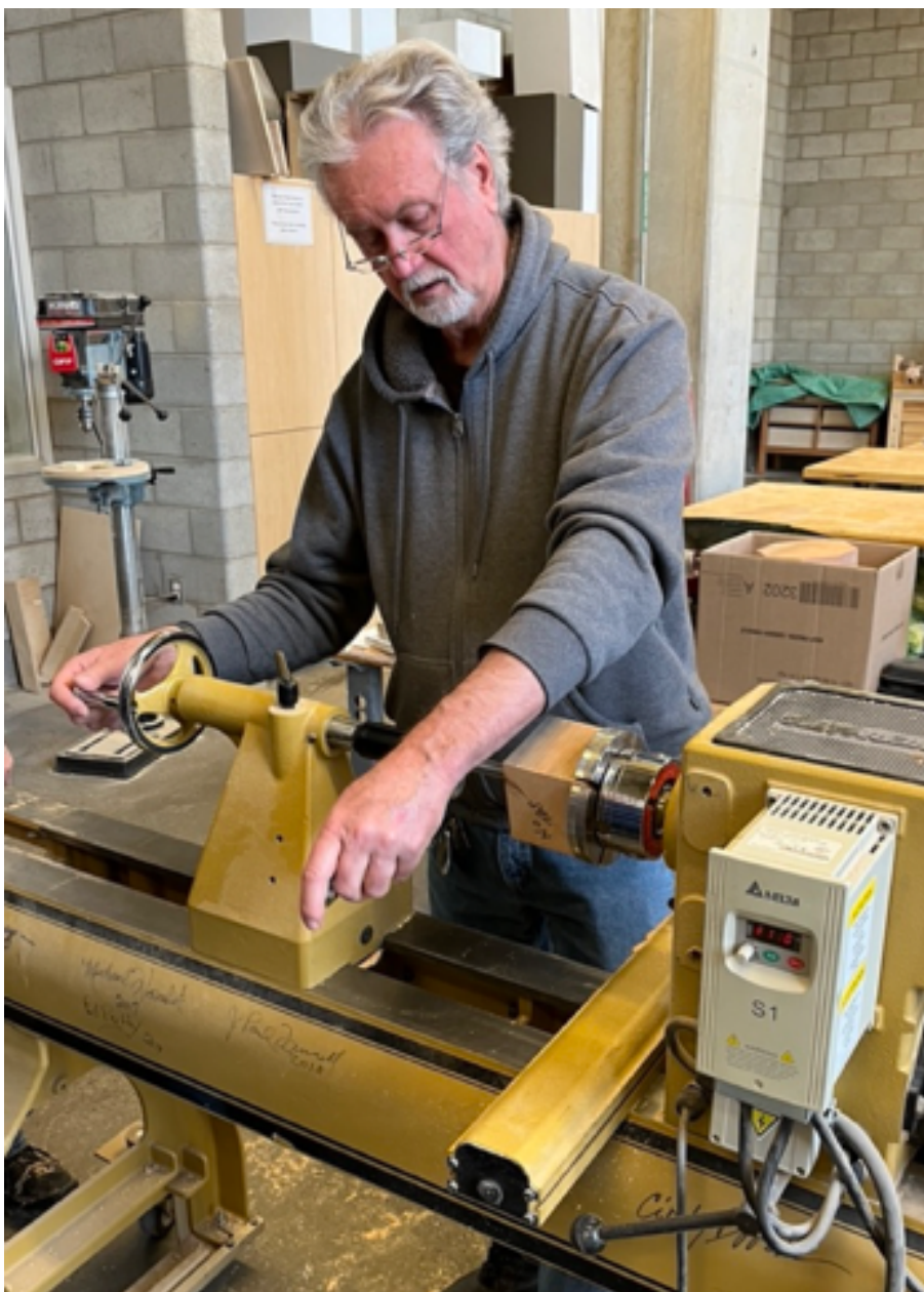
Earl Stamm controlling the tailstock pressure while turning the tap with a wrench.
