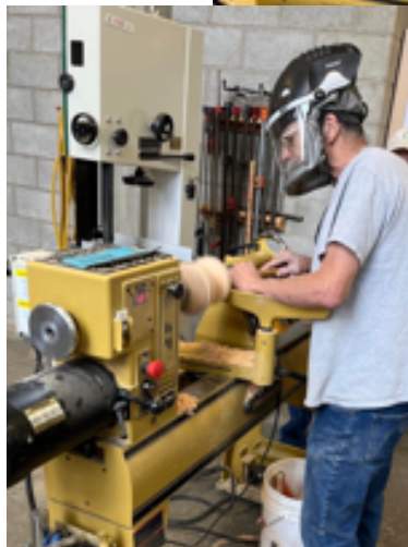
Ron Kisko trims the eccentric. You can see the wobble on the spinning piece.
