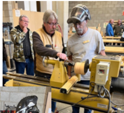
Steve measures Ron Kisko's practice piece. Notice the blank is completely off centre on the face plate.
