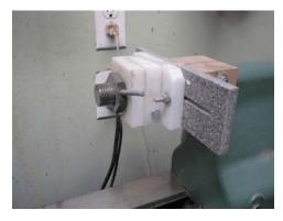
8 threads per inch, the turning mounted in a chuck is screwed onto the tail stock assembly.
