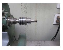
The thread cutter is made from a key way cutter ground to 60 degrees. The key way cutter is from Busy Bee & the cost is around \$14.00. I ground the cutter 60 degrees with an angle grinder chucked in the head stock and turning backwards
