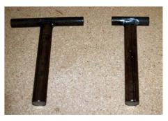
The following tool post is very specific in its purpose. It is simply a tool post with the top notched out and is used when parting off a bowl, etc. The wings keep the parting tool from sliding of the tool rest and because it is so small I can get in very close to the cutting area.
