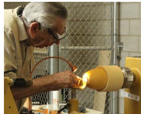
working on base of hollow form in jam chuck
