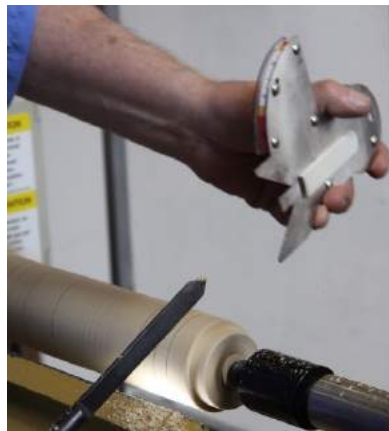
A Gilbert Caliper can simplify establishing the right diameter
