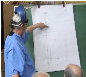
Spindle design, Always use a diagram and measuring stick for spindles - mark the highs and lows
