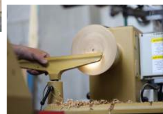
Ed has LED lights with magnets under the tool rest which shine right where the tool contacts the spinning wood
