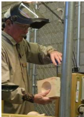
making a safety block to hold spindle for bandsawing
