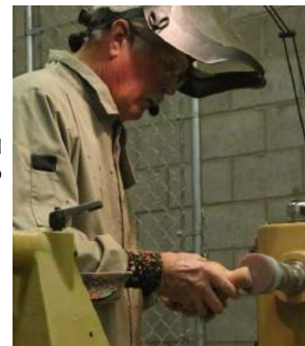
Sanding with a lathe mounted sanding pad
