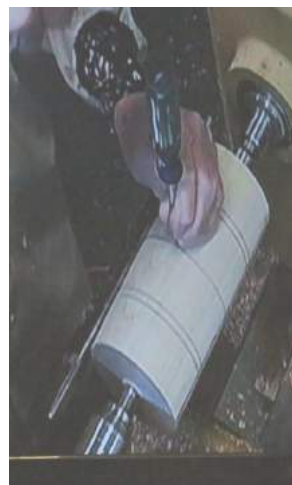
Centre punch the bottom of the bowl
