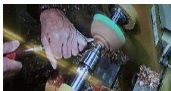
Jam chuck the hollowed cup and cut off the tenon
